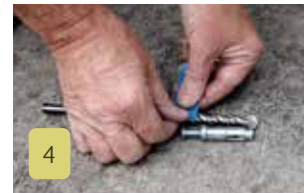
4 Using tape, mark your drill bit to the depth of your screws plus an allowance. Before you start drilling make sure that you clean the area. This will help ensure proper contact and make it safer to work around.
