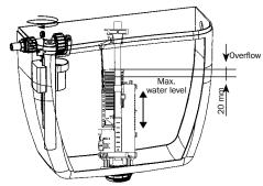
To adjust the water level of the short flush, slide the cursor along (j). Immerse the cursor of 40 mm.
